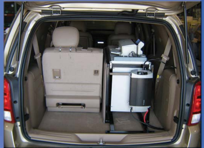
Invertor and power strip for printer
